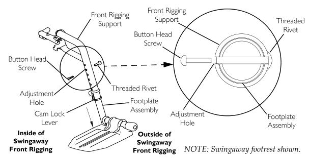
FIGURE 4.3 Bolt-In-Place Height
